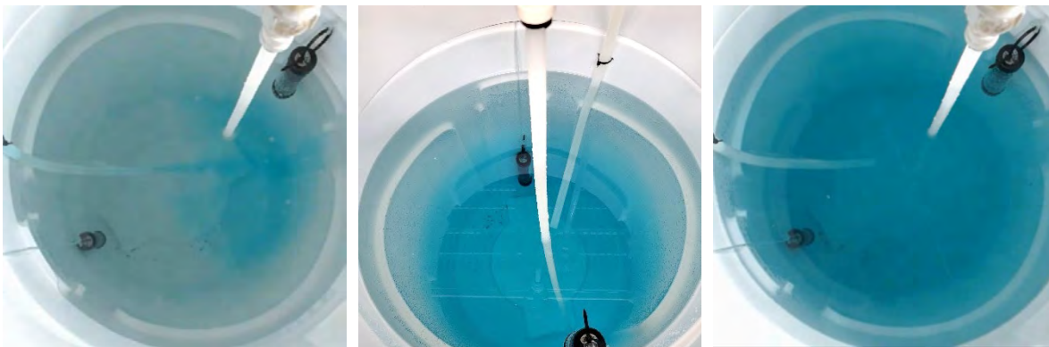
Figure 3-1. Chamber During Mock Test Dye Study: Alkaline Sample Dispersed (Left), During 5-Min Exposure (Middle), and During 3-Hr Flushing Period (Right)
